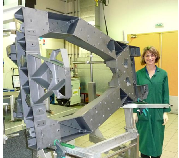
Figure 12. The main structure of Sentinel-2 MSI
